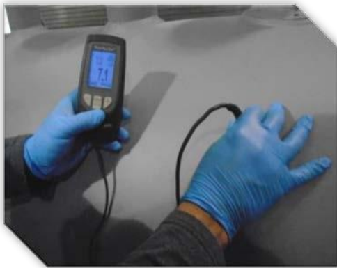
Paint Coating Inspections
